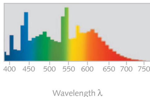
Daylight spectrum of a Biolum<sup>®</sup> fluorescent lamp. The radiation is very evenly distributed over the entire visible range.
